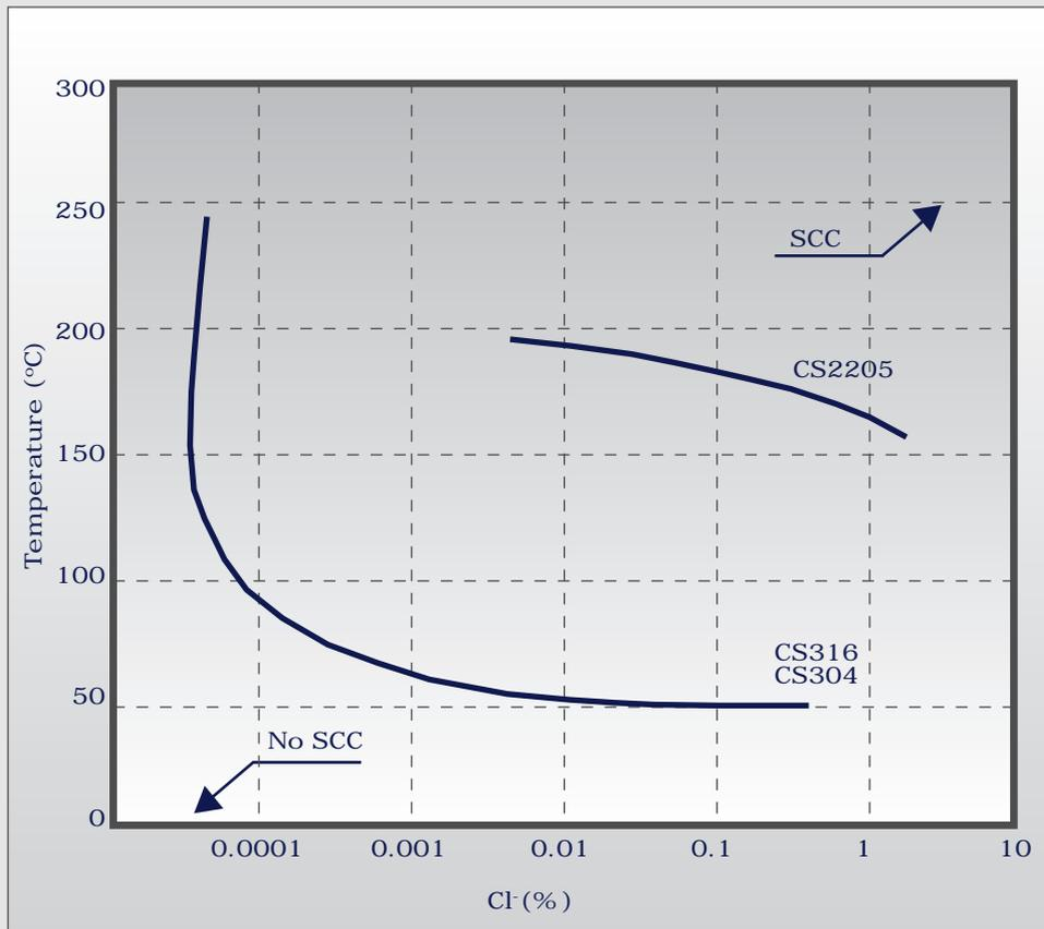
Resistance to Stress Corrosion Cracking (Laboratory results).
